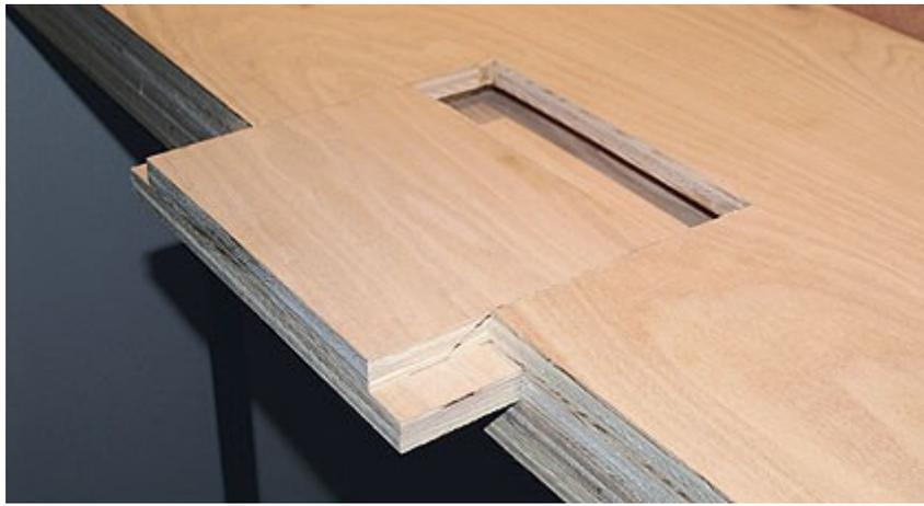
Fashioning the dovetailed cavities for the inserts requires some careful chiseling and filing in order to make them a neat fit with no gaps but not so snug that they are difficult to remove. Here the bench is seen with its component layers clearly visible, inserts in various stages of completion, the front facing partly applied.
