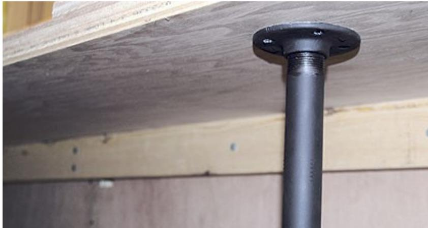
The legs are steel pipe, cut to length and threaded into flanges on both bench and floor. This allows the bench to be leveled, then bolted firmly to become rock solid.
