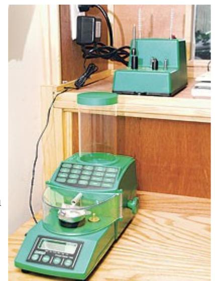
The RCBS ChargeMaster combination digital scale and powder measure. The ChargeMaster and case-prep center (behind) normally live on the shelf above the bench, out of the way but instantly available.
